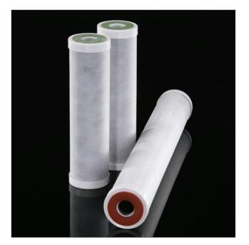
CARBOFLOW MX cartridges are offered in both high efficiency and general grades. They consist of bituminous coal sourced carbon, extruded together with an FDA listed thermoplastic binder, to produce an extremely porous yet rigid structure.
