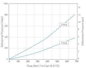
For A size filter, multiply dP by factor of 3 at same flow
