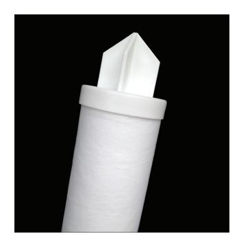
Graded density, high porosity, SPUNFLOW QN filter elements are manufactured from thermally bonded Polypropylene microfibers. Offering high throughputs, low pressure loss, high holding dirt capacity and long on-stream life, the bonded fibre construction minimizes any possibility of fibre migration and is rugged enough to resist particle shedding, even under pulse conditions.
