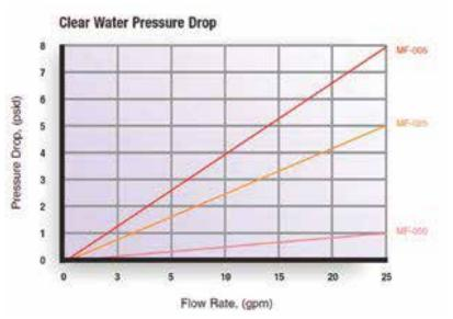
This chart show the Vorex® filter cartridge pressure drop as related to flow-rate per 10 inch cartridge length. Results may vary in actual service.
