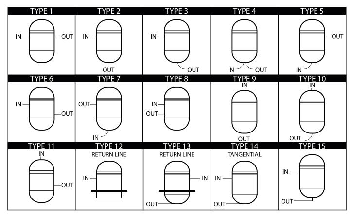
NOTE: Inlet and outlet nozzles are shown in general positions. They can be rotated or relocated to meet customer requirements.
